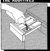
Pour the softener, if required, into the compartment marked \$\mathbb{8}\$ ; do not exceed the MAX level.
